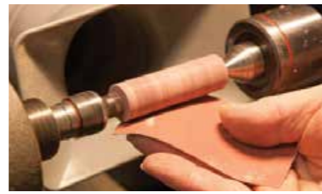
Sanding with the lathe running should be followed by hand sanding along the grain
