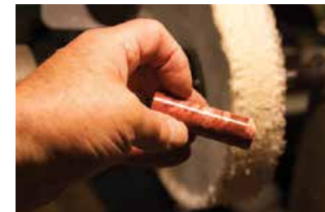
Buffing can produce a high gloss finish on acrylics, hard finishes and stabilised wood
