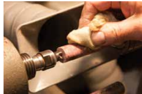
Cleaning away sanding dust between grits prevents scratching from any remaining coarser grit particles
