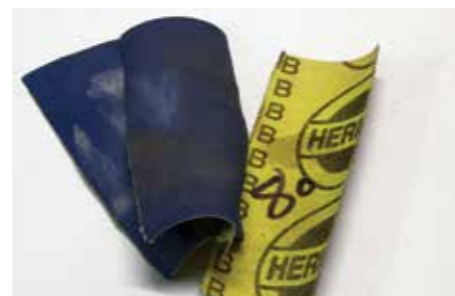
Strips of cloth-backed, aluminium oxide paper are a popular choice but remember to write the grit grade on the backing to avoid confusion
