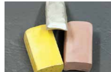
Compounds for buffing wheels come in a variety of grades from coarse to very fine. A separate buffing wheel should be used for each grade
