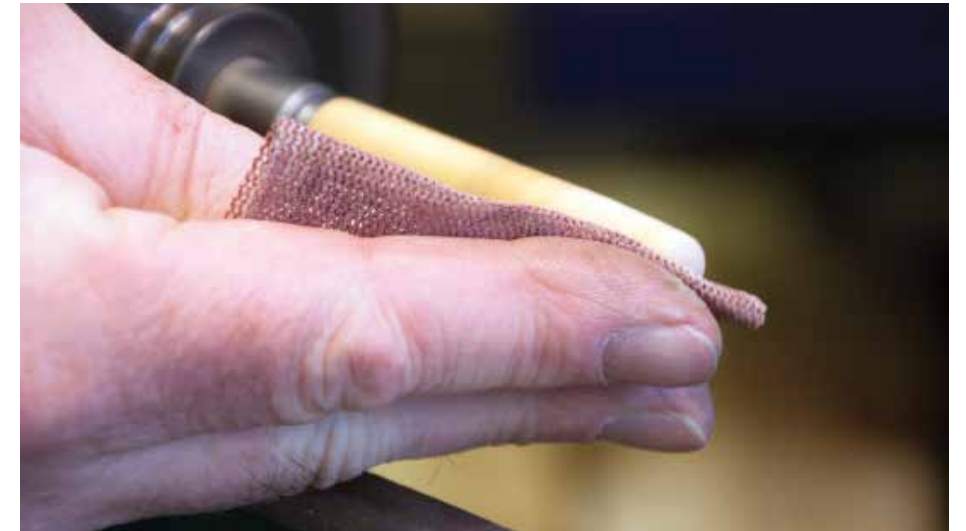
All finishing work can be completed on the mandrel
