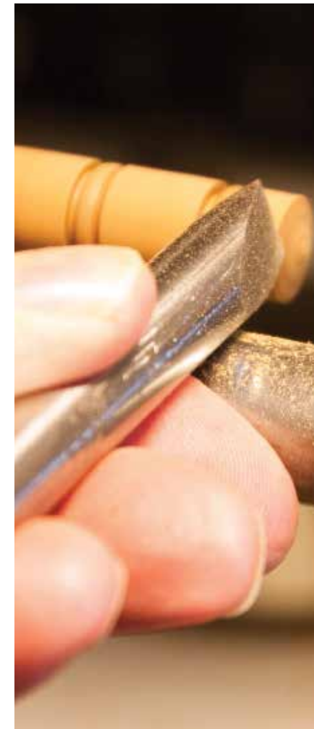
Cleaning up the parted off end with a skew chisel
