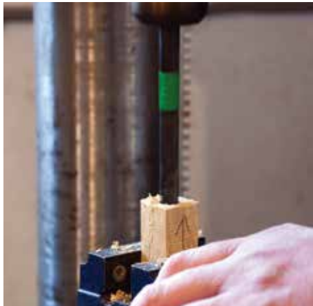
Mark the drilling depth with tape around the bit
