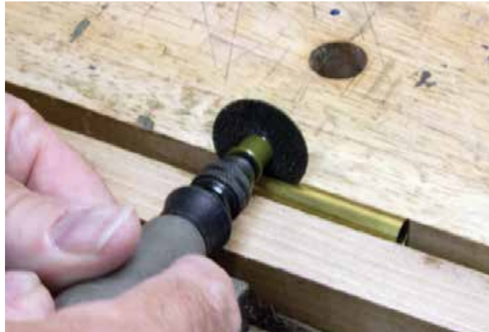
Slicing a slightly too large tube along its length can help to match the diameter of your tricky pen
