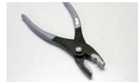
These plumber's pliers are ideal for pen dismantling, thanks to their soft jaws
