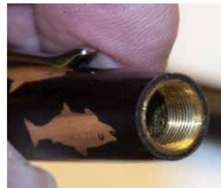
Here, it is not possible to remove the threaded insert from the tube without removing the mechanism first
