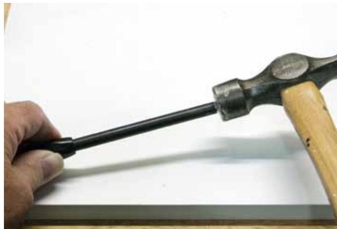
Using a suitably sized transfer punch to drive the components out of the tube
