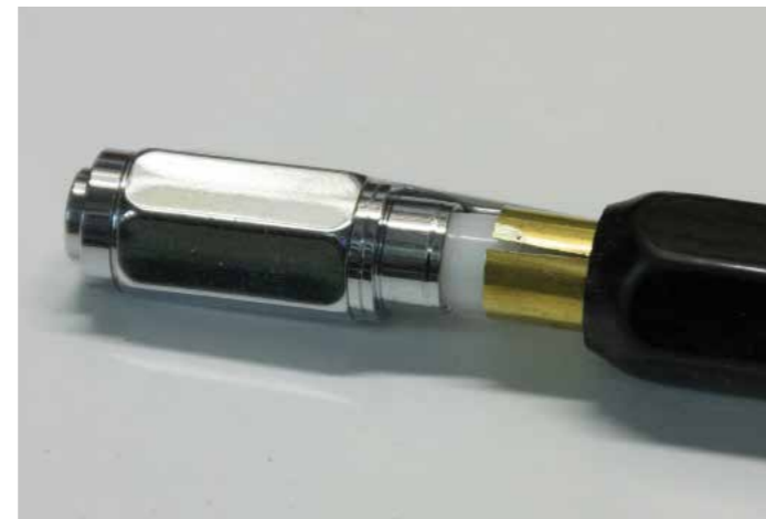
The slit tube slips over the plastic parts but is still able to contact the end of the metal components
