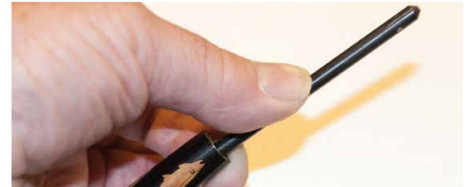
A suitably sized punch, a hammer and revolving the blank will allow it to release without damage
