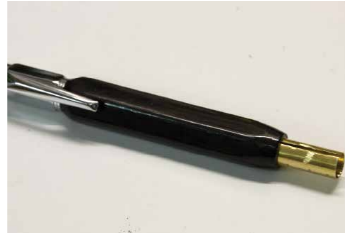
A slit tube has been inserted into the open end of a click pen once the writing tip has been removed
