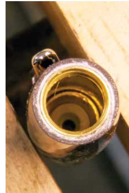
The outline of the brass components at the top of the pen surrounding the nylon click mechanism
