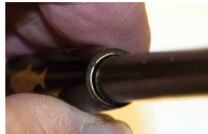
The components at the other end of the tube can be removed using a suitably sized punch
