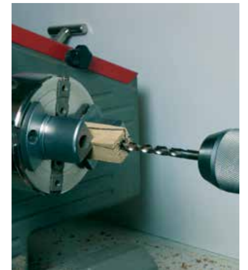
A dedicated pen blank chuck facilitates drilling on the lathe
