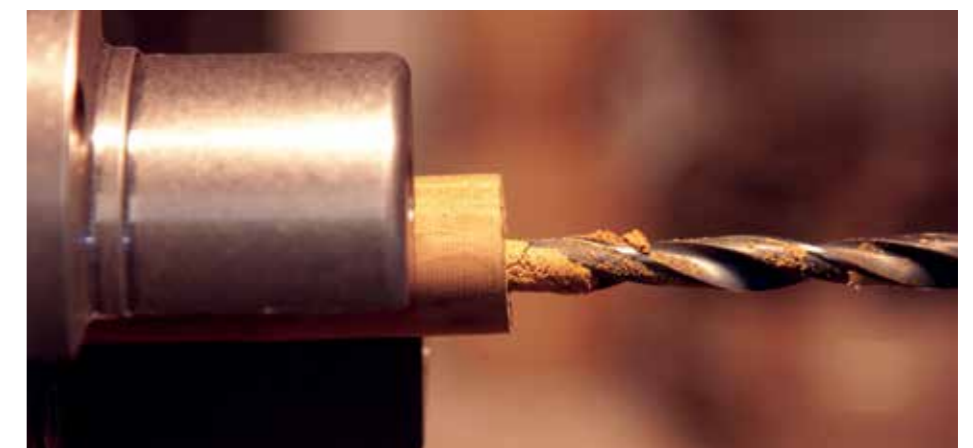
Withdraw the bit frequently to prevent clogging of the flutes
