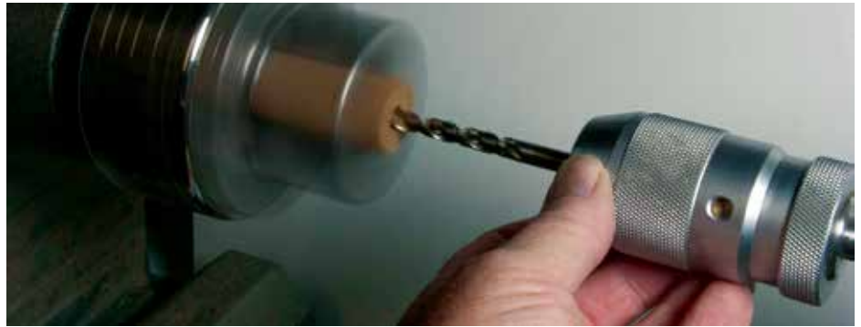
Grip the chuck lightly when withdrawing to avoid disengaging from the Morse taper
