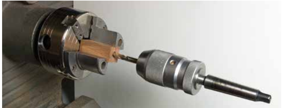
If the chuck is allowed to disengage from the Morse taper it may become a potential projectile
