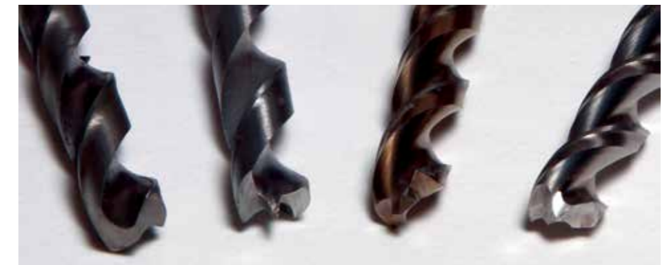
FROM LEFT TO RIGHT: Jobber bit; lip and spur bit; bullet tip bit – pilot point bit – and Colt pen bit
