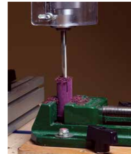
Using a pillar drill and drill press vice will enable accurate drilling
