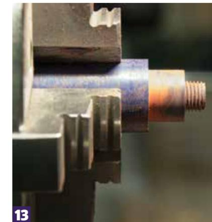
**13** Cut the threads right up to the face of the work by reversing the die in the holder. There is no need for a recess behind the threads as the clip will provide the necessary clearance. This part can then be parted off using a thin parting tool. Take care not to lose this small component by holding it lightly with one hand while parting off, but do keep your fingers clear of the very unforgiving engineers' jaws
