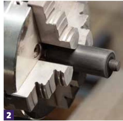
**2** Using the methods outlined in my previous articles, cut the threads on the spigot using an M10 x 1.25 die. This is quite a large size and a coarse thread, but the next size down in a standard set of taps and dies is usually M8, which does not leave sufficient clearance to accommodate the 6.5mm diameter bore required for the body of the refill. The size makes for a chunky pen and the coarse thread is concealed when the pen is in use
