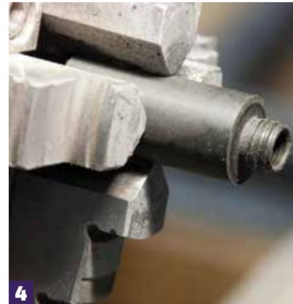
**3** Drill out for the refill, first drilling right through at 3mm diameter, then to 4.8mm and then 6.5mm to the precise depths shown in the drawing. This will ensure a good fit of the refill in the writing tip of the pen. If your tailstock quill is calibrated you can use this to measure the depth, otherwise mark the drill with tape
