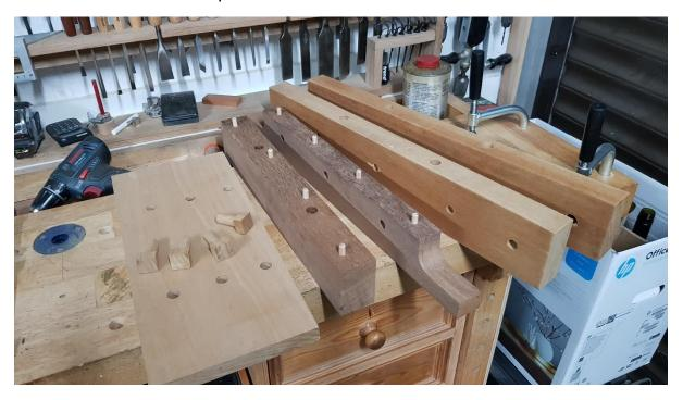
The front support has extended ends so the vice can be clamped to the bench with hold downs or cramps. The two supporting pieces are glued and dowelled to the "bench top".
