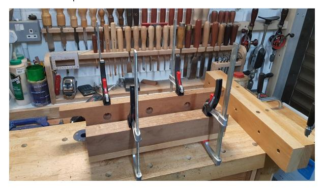
The rear jaw is bolted to the body of the vice with three M12 bolts so it can easily be replaced if and when it becomes worn or damaged
