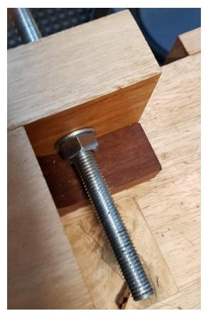
Normally the jaw opening required will only be a couple of inches, but I left sufficient threaded rod to the rear of the jaw so that it can be extended if necessary, to increase the jaw capacity.
