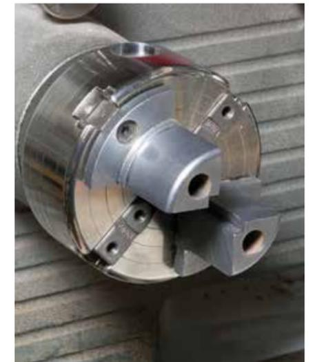
Dedicated pen jaws can be used to hold the blank for drilling on the lathe
