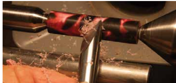
Using a skew chisel
