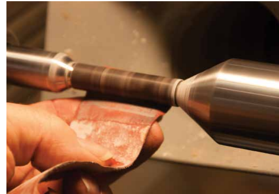
Wet sanding keeps the blank cool
