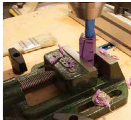
Stop drilling when the tape just touches the blank
