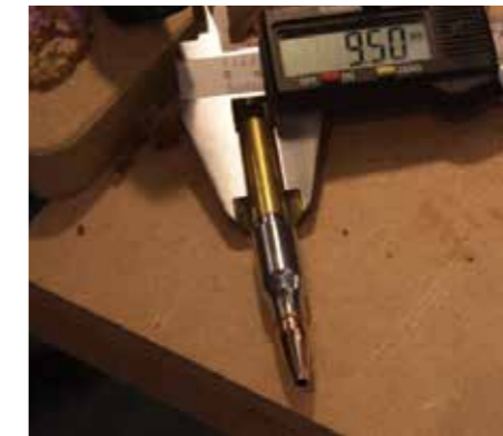
Measure the thickness of the walls – component \varnothing – tube \varnothing – to determine whether tubes need to be painted
