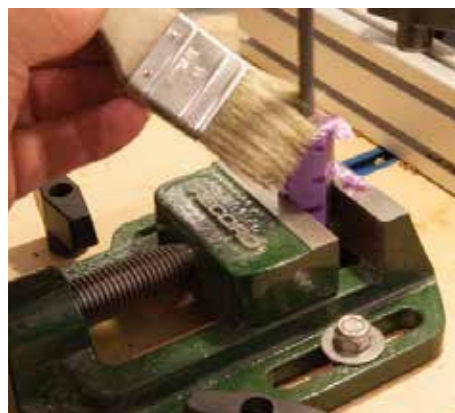
Regularly withdraw the bit and brush away swarf
