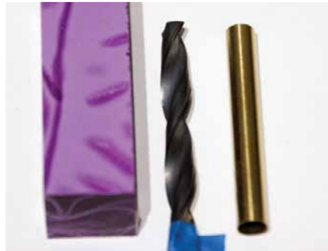
Drill bit and blank prepared to drill short of breakthrough
