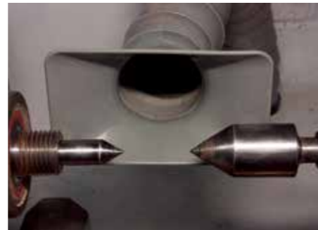
An extractor inlet placed near the work will draw fumes away from the user
