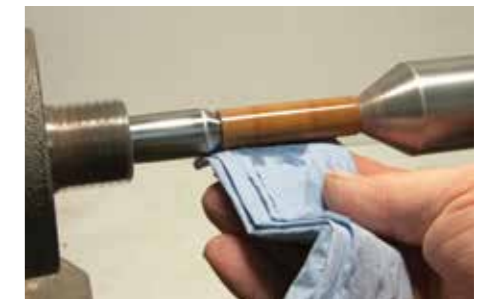
Keep the applicator moving to avoid sticking
