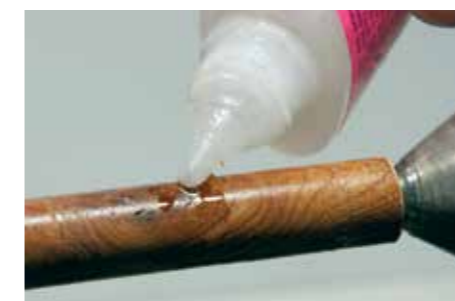
Thin CA can be used to repair voids in burrs or chips in acrylics
