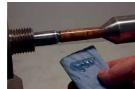
A line of CA applied to a paper towel is wiped quickly over the blank
