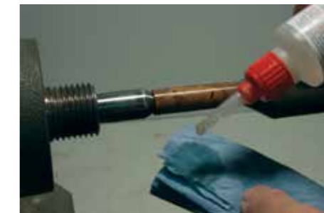
A drop of BLO may be applied to the towel before a few drops of CA
