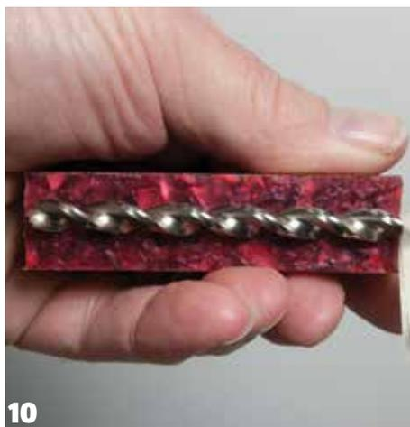
**3** The barrel is longer than most pen blanks so will have to be drilled on the lathe since most pillar drills will have insufficient travel. Using a chuck fitted with pen blank or pin jaws and a long drill bit in the tailstock chuck carefully drill out for the brass tube.
