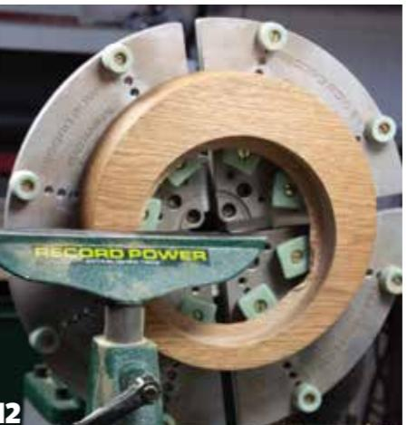
**5** Now sand the prepared areas of the blank through the grits to a finish as it will be difficult to re-mount the blank to do this at a later stage. A cordless drill with sanding pads will minimise radial or annular scratch marks. Do not apply a finish at this stage as it may inhibit the effectiveness of the wood glue later in the project.
