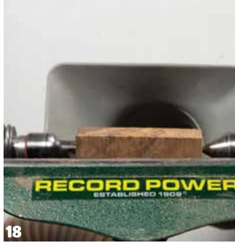
**18** The final part of the job is to make and fit the feet. You could turn these from a single walnut spindle blank but I used offcuts from two nicely figured pen blanks. First turn to a cylinder between centres.
