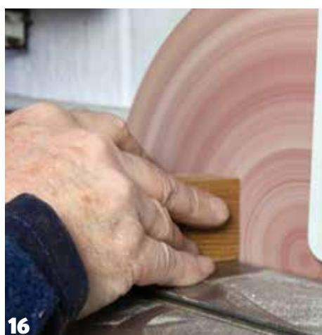
**16** True up the ends of the cradle section on a disc or belt sander. They can then be sanded through the grits by hand to a finish.
