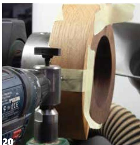
**20** The holes in the body are also drilled using the same jig with the work mounted on a scroll chuck. Take care to mark the hole positions carefully. I used masking tape to avoid pencil marks on the finished work. Once the feet are glued in place using 6mm dowels cut to length the finish of your choice can be applied. I used Natur-Öl finishing oil from Drechseln und Mehr. ●
