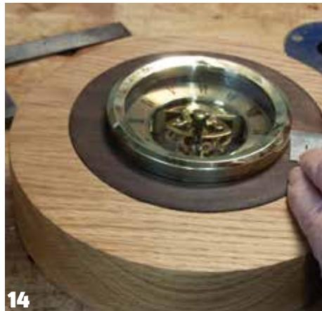
**14** With the clock mechanism inserted and the surround fitted to the outer section, carefully mark the position for the part that will be removed. This should be on the centreline of the clock face.
